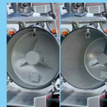
Movable partition for capacity increases
