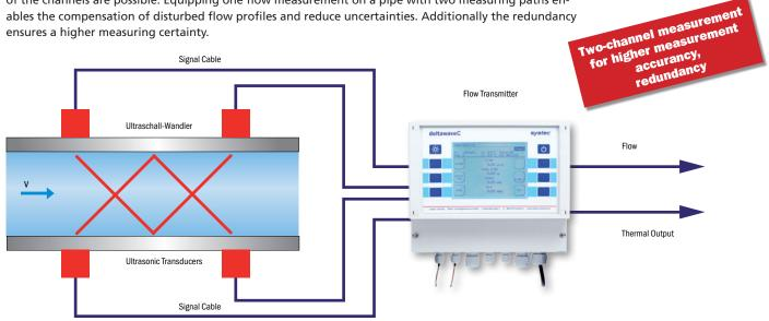
Compensation of distrubed flow profiles with two-channel measurement
