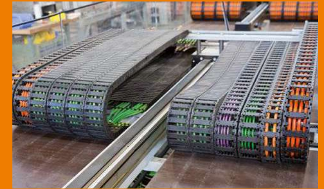
Bend factor test, 76 million strokes at 9.4 x d
