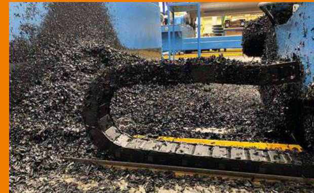
Enclosed energy chains for reliable protection against dirt and swarf
