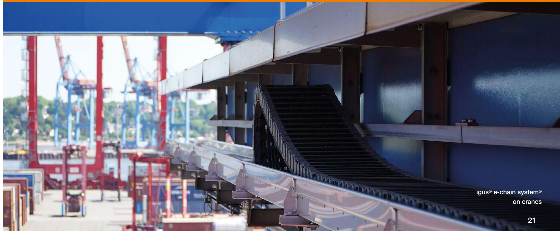
Enclosed energy chains for reliable protection against dirt and swarf
