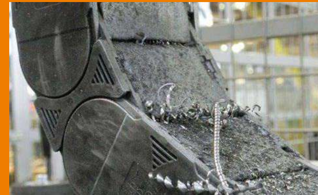
Swarf test, 100% swarf-resistant
