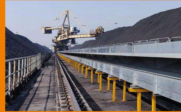
Extremely long travels with rol e-chains® (here 700m)
