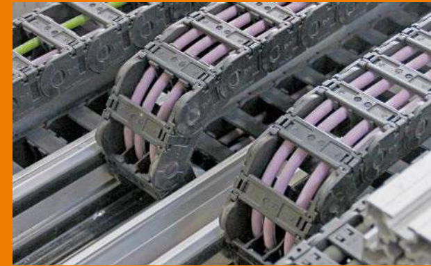
Cable test, more than 80 million strokes
