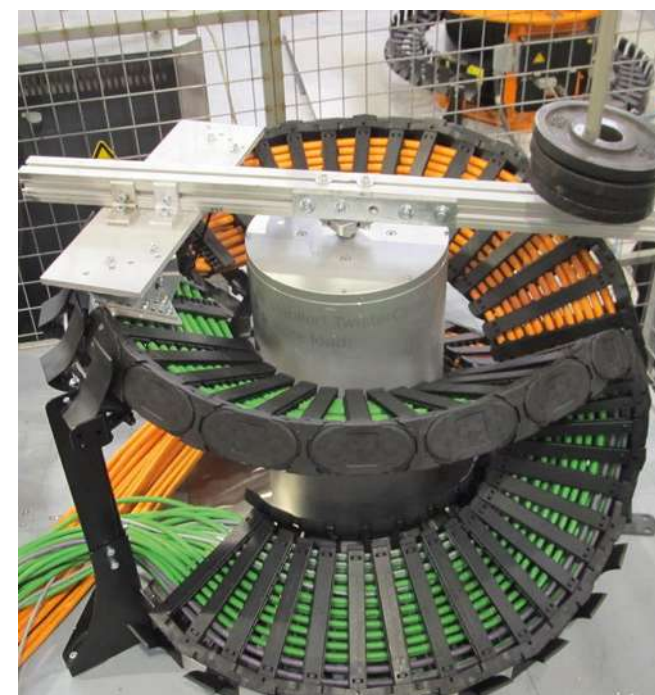
Rotary movement tests in very demanding chain applications using igus® twisterchain®
