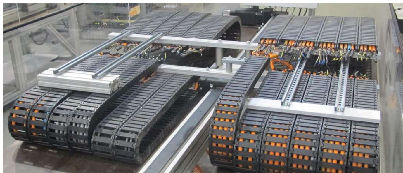
Linear chain tests of all chainflex® cables with different radii and travels
