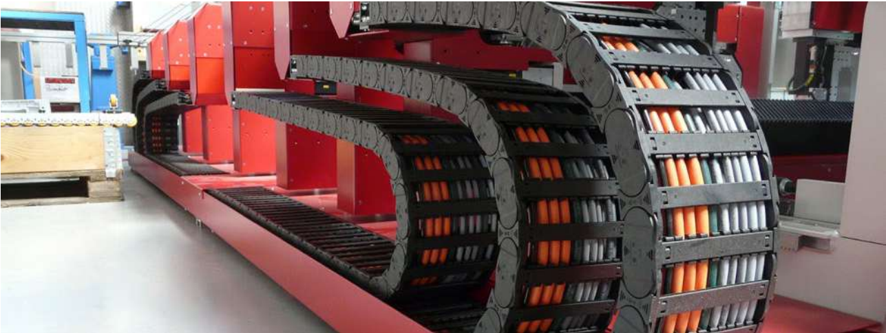
Drilling machine for wooden plates equipped with latest hybrid cable technology with Hiperface DSL
