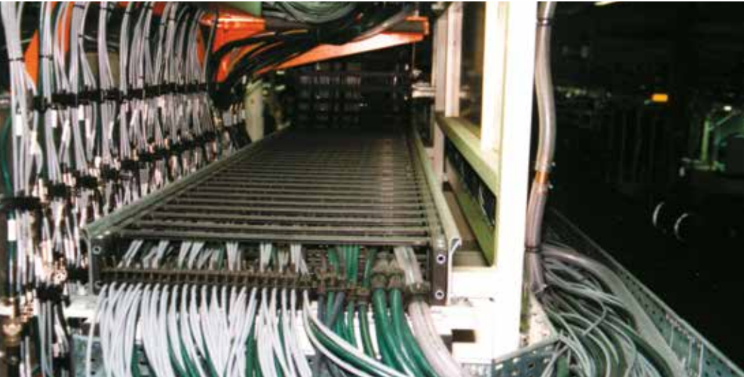
Chainflex® CF5 and CF6 control cables (green) as well as CF211 measuring system cables (gray) in a screwing station of a motor factory. E-Chain®: System E4/00 with chainfix clip strain relief devices
