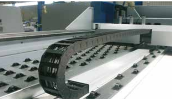
Chainflex® CF130.UL for woodworking. E-Chain®: E4/light
