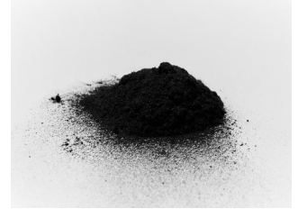
Activated carbon For removal of hydrocarbons, chlorine or other unwanted dissolved components by adsorption
