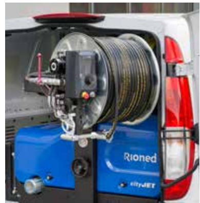
Wide 180° pivoting hose reel for max. 140 metres of 1/2"hose
