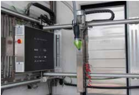
In this 3D printer, a linear robot is used, in which the x- and y-axis have been implemented with drylin® toothed belt units
