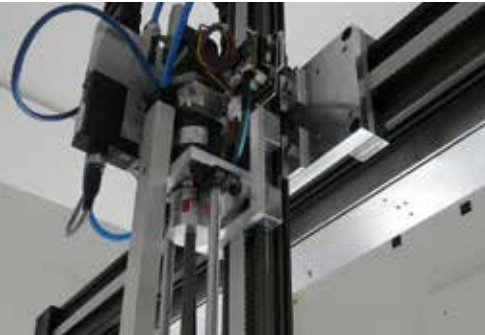
drylin® toothed belt axes are used on the three linear axes of this Pick & Place system
